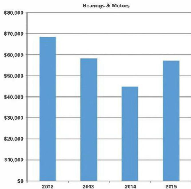
Fig. 3. The cost of bearing and motor replacements decreased due to data collection and predictive maintenance.
